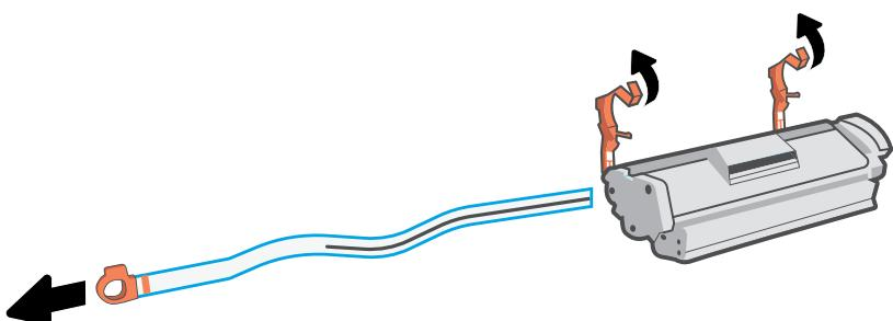
**EN** Remove the orange guides, tape, and pull the tab to remove the protective film.
