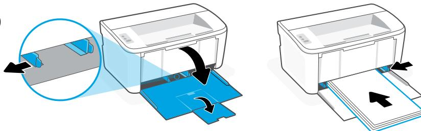
**EN** Open the input tray and slide out the guides. Load Letter or A4 paper and adjust the guides.
