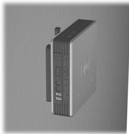
Figure 5-7 Thin client mounted on wall
