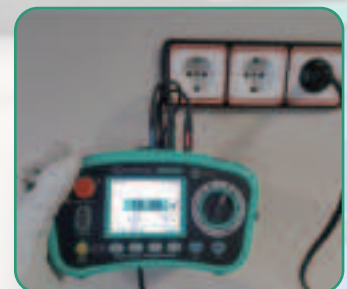
Loop test from a wall socket
