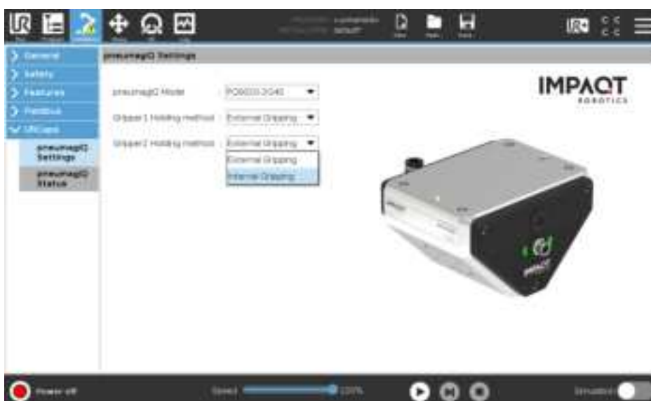
Figure 7: In the installation tab, under URCaps select the Tool Gripping mode for pneumagiQ
