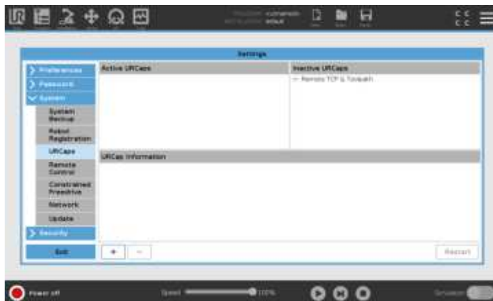
Figure 2: Use the '+' button at the bottom left to install the pneumagiQ URCap
