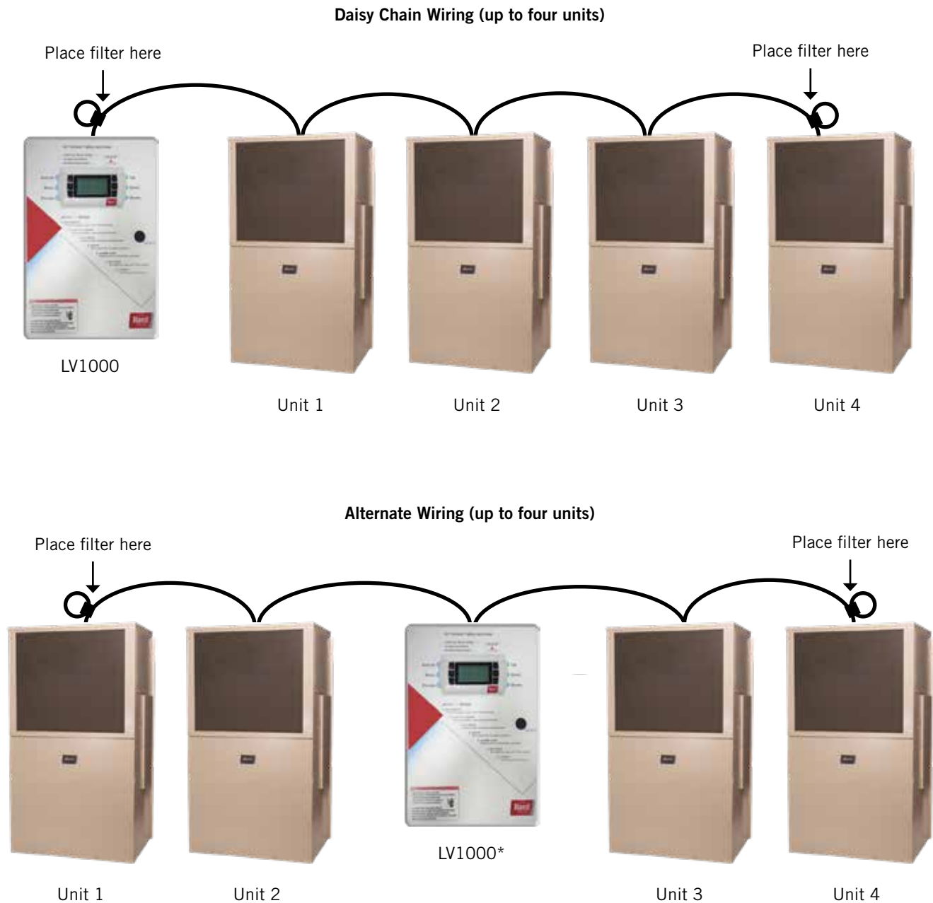
FIGURE 26 Placement of Communication Wire Filters (Daisy Chain and Alternate Methods)
