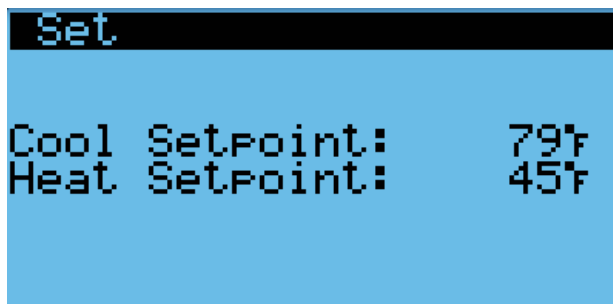
FIGURE 19 Cool and Heat Setpoints
