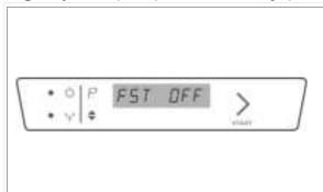
**Fast start (FST):** starts the dishwasher in less than the standard time; leads to higher water consumption for the first cycle start.
