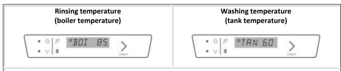
**Warning:** The tank and boiler temperatures shown on the display may be different from the actual temperatures by a few degrees, especially in transient phases (just after the FILL is completed, just after the end of the cycle, etc.) due to the inertia of the measurement probe.
