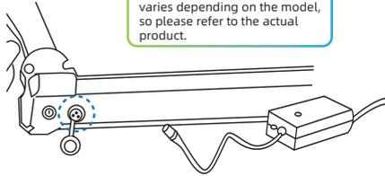
1. Open the charger port cap and connect it to the connector of the charger and connect it to the household outlet.
