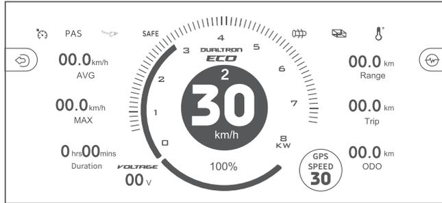
The new system for the EY3 screen LCD only displays the service symbol when the scooter breaks down. In this case, you need to check the APP to view the specific error code. The APP will display the following four error symbols. When there is a fault, please contact after-sales service or an authorized dealer.
