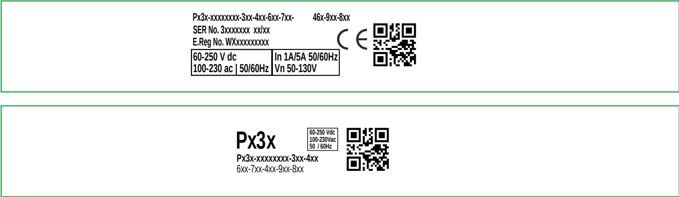
Fig. 5-1: Example of the type identification label of a device from the Easergy MiCOM 30 family.
