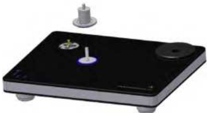
Pic. 6: Fitting the bearing upper part
