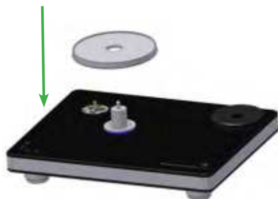
Pic. 7: Setting the sub-platter
