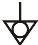
**WARNING:** Risk of electric shock. If the SPA is placed at a distance of less than 118 inches from metal surfaces, then each metal surface is permanently connected by a (at least 1mm<sup>2</sup>) solid copper conductor to the wire connector on the grounding terminals located at the bottom of the power box that is provided for this purpose.
