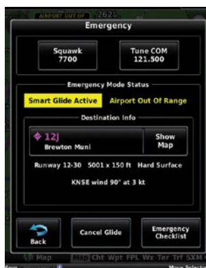
Airport Out of Range (Emergency Page)
