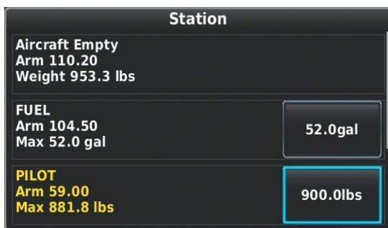
Loading Limit Exceeded
