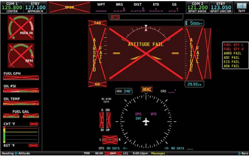
G3X Touch System Failure Annunciations
