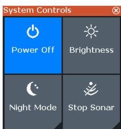
Press the power key once to access the **System Controls** dialog and:
