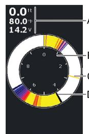
The flasher application shows a raw, live sonar view commonly used in scenarios such as ice fishing and vertical jigging.
