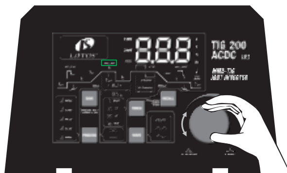
Step 2: Rotate the parameter knob to adjust the welding current to the desired level.
