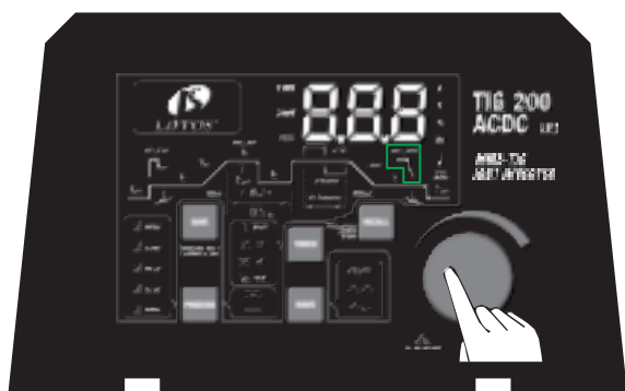
Step 5: Press the parameter knob to select the ARC-Force mode* .
