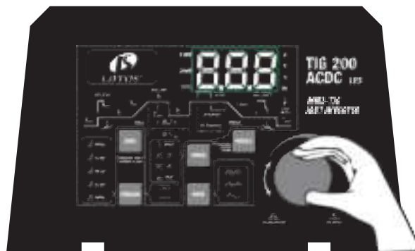
Step 4: Rotate the parameter knob to select the desired serial number, then wait for 3 seconds to Recall the saved settings.
