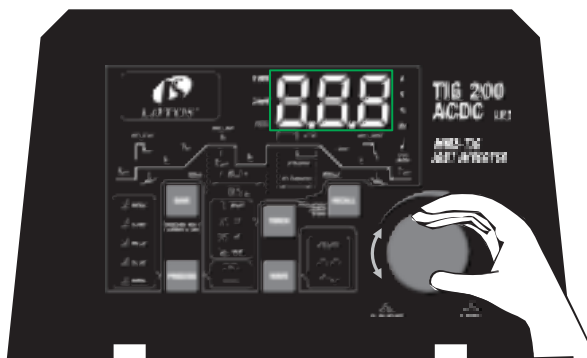
Step 35: Rotate the parameter knob to select a number, then wait for 3 seconds to SAVE the
