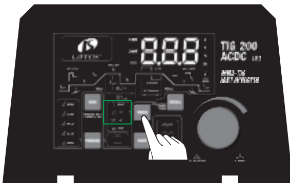
Step 19: Press the TORCH button to select the 2T/4T/SPOT function.
