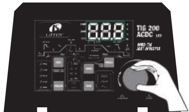
Step 12: Rotate the parameter knob to adjust the Pre-Flow time.(0.1-3.0S)
