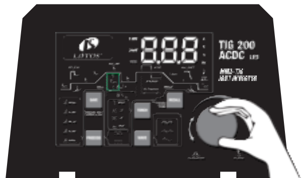
Step 20: In SPOT mode, press the parameter knob to select the SPOT function, then rotate the knob to adjust the SPOT time.
