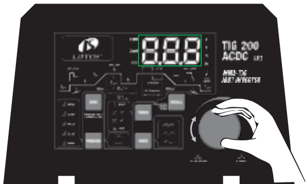
Step 14: Rotate the parameter knob to adjust the Start Amps Time.(0-10S)
