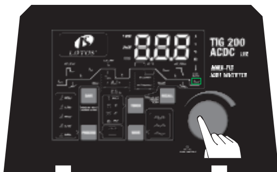
Step 9: Press the parameter knob to select the Post-Flow function.
