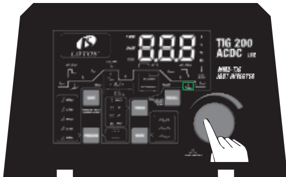
Step 7: Press the parameter knob to select the End Amps Time function.
