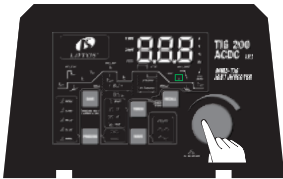
Step 5: Press the parameter knob to select the End Amps function.
