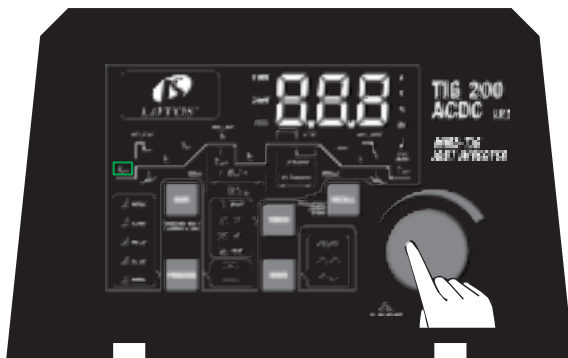
Step 11: Press the parameter knob to select the Pre-Flow function.
