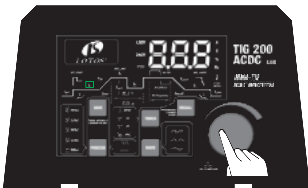
Step 15: Press the parameter knob to select the Start Amps function.
