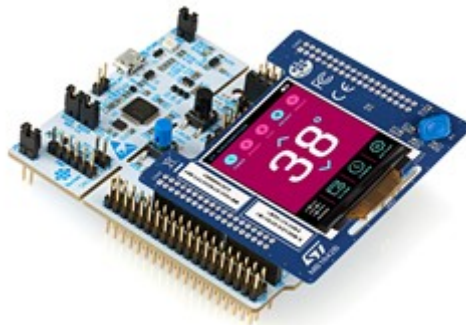
Figure 1. X-CUBE-DISPLAY running on NUCLEO-G071RB equipped with X-NUCLEO-GFX01M1
