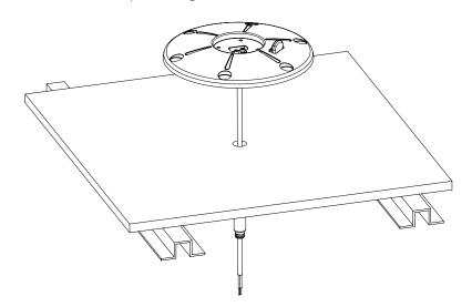
2. Once floor base location and wire entry hole position is located, Using the template, mark the location of the wire entry hole and mounting screw holes. The wire entry hole should be sized to 3/4" to allow in-line fuse to pass through the hole. Mounting screw holes should be sized appropriately for mounting floor material and screw style. #12 screws are recommended for installation. Drill holes appropriately.
