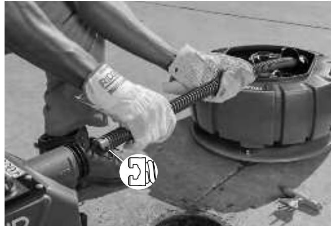
Figure 7 – Inserting Cable Into Front Of Machine
