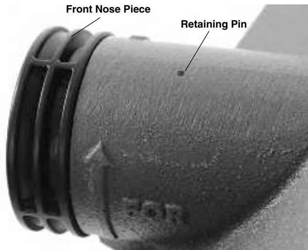
Figure 21 – Front Nose Piece Change Out
