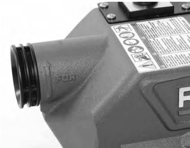
Figure 10 – FOR Machine Rotation Marking
