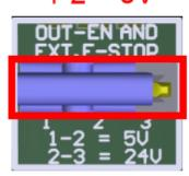
If used a power supply of 24VDC and in the output of terminal de EN and EXT E-STOP wwork with 24V, set jumper as sample in the image.
