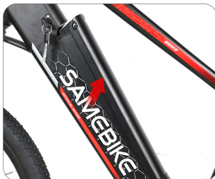
Remove the battery upwards
