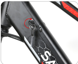
Turn the key clockwise to unlock the battery lock
