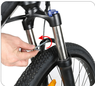
Loosen the set screw counterclockwise
