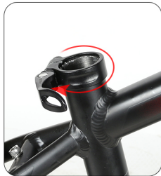
Loosen the quick release lever according to the direction
