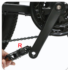
The pedal "R" is installed on one side of the chainring, and "L" is opposite to the chainring
