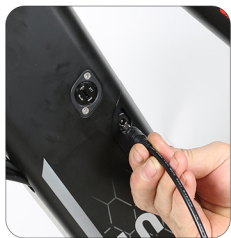
Plug the charger into the power hole
