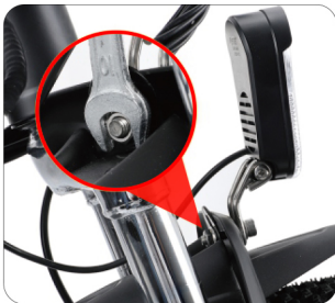
Put in and tighten the headlights and front fender respectively
