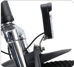
Install the headlights and front fender
