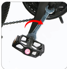
Tighten the right pedal "R" clockwise
