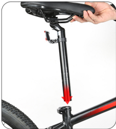
Insert the seat tube in the direction
