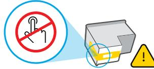
**EN** Remove the orange caps and tape from the printheads.
