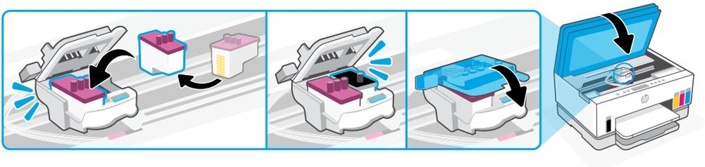
**EN** Position the electric contacts facing the printer, insert and click into place. Close the printhead cover and the ink access door.
