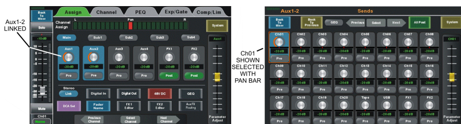
Figure 4.7c: Aux1-2 are linked, Ch01 sent to Aux1-2 and assigned to Main mix
