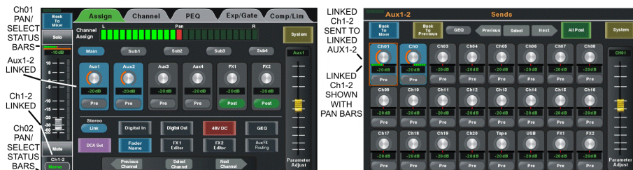
Figure 4.7d: Ch1-2 Linked, Aux1-2 also linked, both can be routed to Main mix
