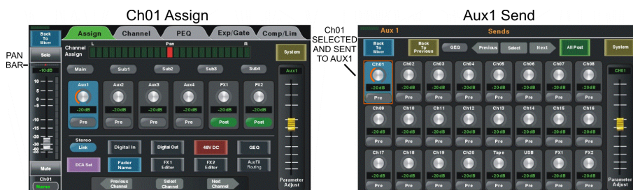
Figure 4.7a: No Linking, Ch01 sent to Aux1 only
