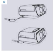
D. Verify that the plug at the si de of the device, at the power supply, and at the electrical outlet are fully Inserted. This will help to ensure that a secure reliable electrical connection has been made.
