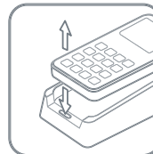
Press the button to lift the card reader out
