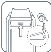
Push down on the ridges to replace the paper roll
