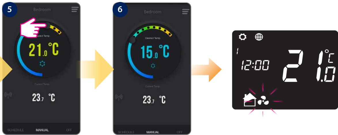
Using the cursor, set the temperature.
