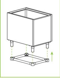
Fully tighten the joint 6 socket set screws.
