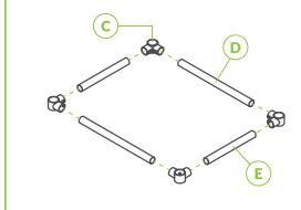
Place ice bin legs into the vertical section of the joint socket.
