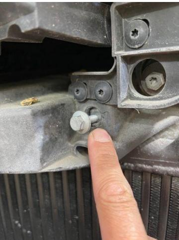
Unbolt the front metal crash bar and you can loosen the opposite side so the bar is loose. You will need to install the intercooler bracket between the bar and the core support.
