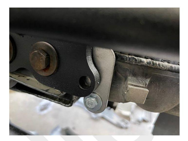
Trimming of the intercooler shroud is necessary based on how much the intercooler is pulled forward. If you do not trim the shroud will come in contact with the bumper and you cannot get it back on.
