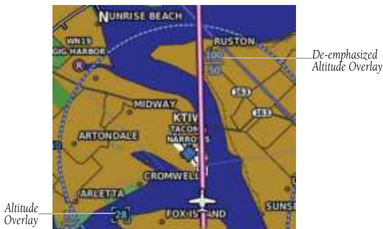
Smart Airspace™ with Altitude Overlays
