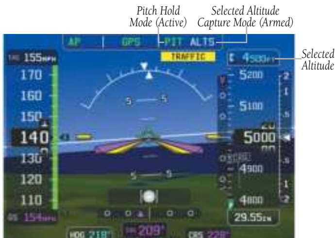
Pitch Hold & Selected Altitude Capture Modes
