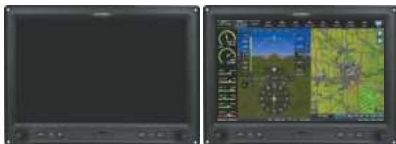
G3X Touch Full-Screen Reversionary Mode (Failed PFD)
