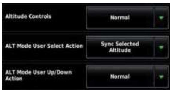
Altitude Controls (Normal)
