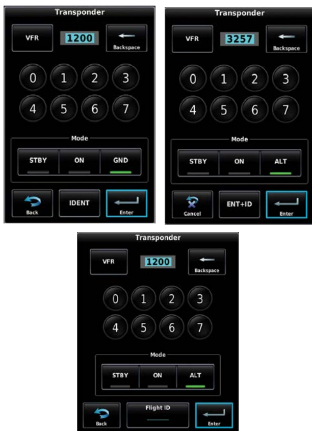
Transponder Code, Mode, and Flight ID Entry
