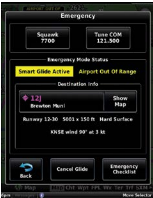
Airport Out of Range (Emergency Page)
