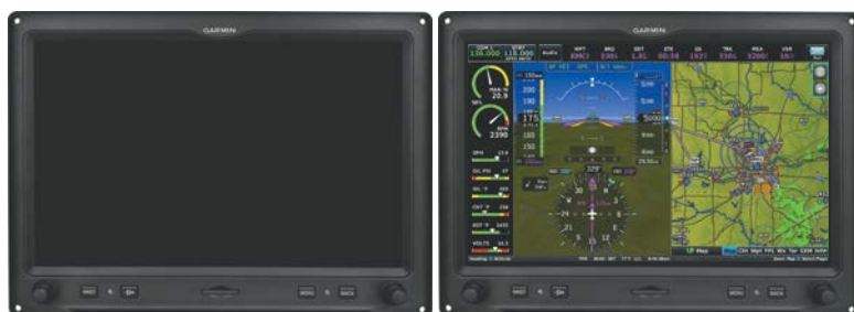
G3X Touch Full-Screen Reversionary Mode (Failed PFD)
