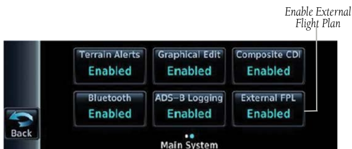
External Flight Plan Enabled (Configuration Mode)
