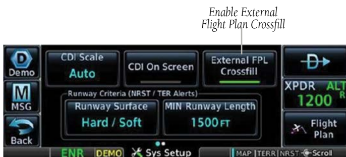
External Flight Plan Crossfill Enabled (Normal Mode)
