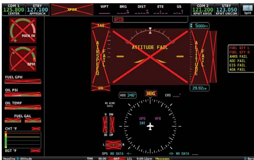
G3X Touch System Failure Annunciations
