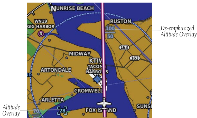
Smart Airspace™ with Altitude Overlays
