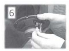
Cut any excess wire to minimize how much will be inside the pod. Connect your speaker. #120998-K65 use the small lengths of wire and red butt connectors that came with your Kicker speakers and connect to the speaker wires in the pods, pos+ to pos+, neg- to neg- #120998 using your own speakers, similar wiring likely came with your speakers. Repeat process for other pod.
