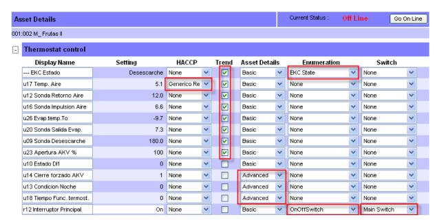
Once one controller has been completed, the work can be saved in a file and restored in other AK-EM 100 projects. It is also possible to copy from one controller to others.
