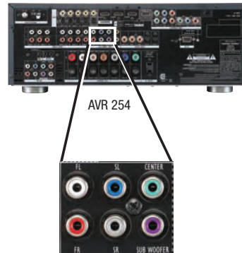
Figure 21 – Connecting a Multichannel Audio Player
