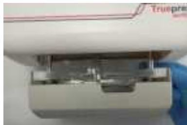
Figure 14: Removal of Replaceable Tray from cartridge holder
