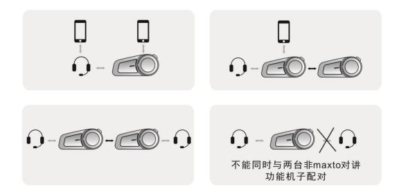
Note: Non-Maxto intercom features are added to the ICEBRKR after the phone is connected
