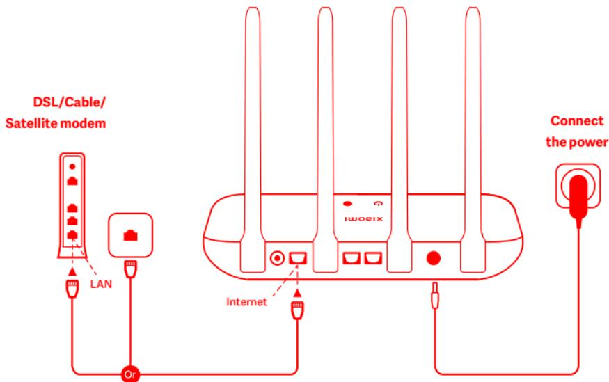
**Power on the router, then connect the Internet (WAN) port to the DSL/Cable/satellite modem**
