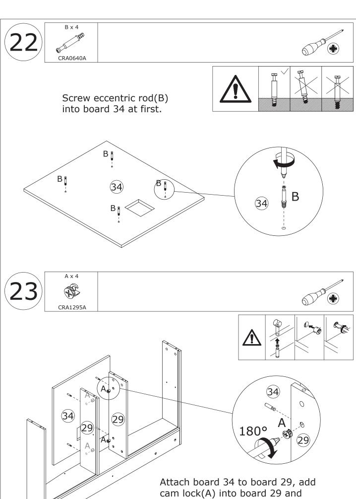
turn clockwise to tighten as shown.
