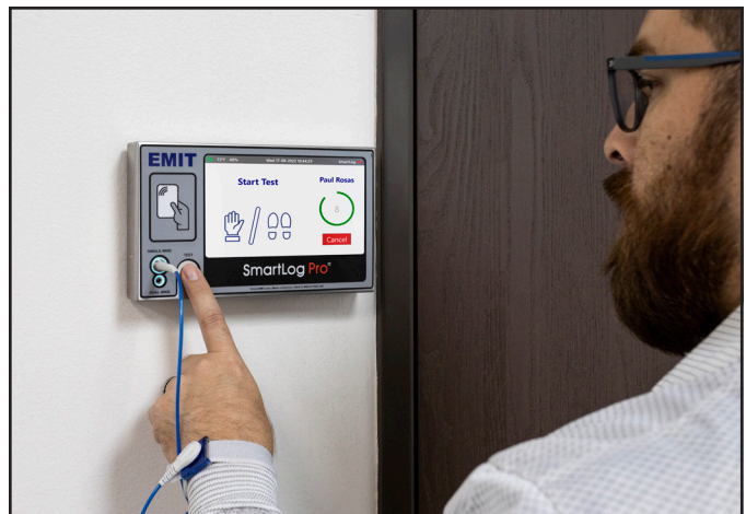
Figure 24. Performing a single-wire wrist strap test
