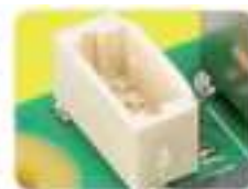
Fan interface with PWM control and tachometer feedback ( 4 pins JST )
