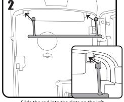
Slide the rod into the slots on the left side of the backpack.
