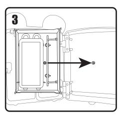
To replace the bed, insert the peg under the bed into the peg on the backpack.
