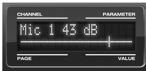
Figure 4-3: The LCD gives you feedback as you turn the TRIM knobs for the two mic/guitar inputs.
