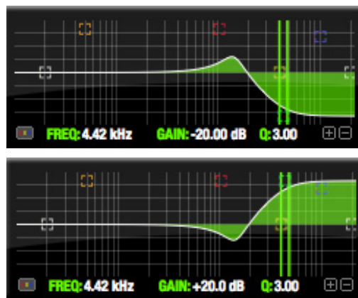
Figure 9-19: Overshoot when high shelf cut and boost is applied.
