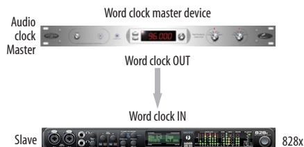
Figure 4-18: Slaving the 828x to word clock. For the 828x clock source, choose 'Word Clock In'.
