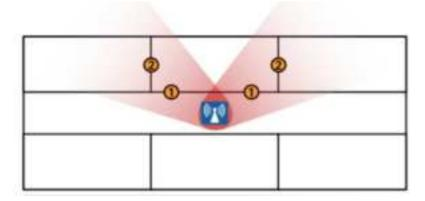
Reasonable placement of APs: Signals pass through a single wall
