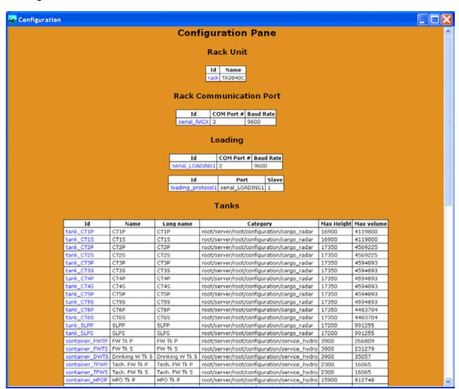
From this window, it is possible to change the name of the processing system, port COM protocol, to allocate characteristics of each tank and allocate characteristics of each radar.
