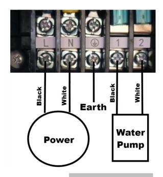
The output of the VDPYCA-65 pump terminal is 110-120V~/60Hz.
