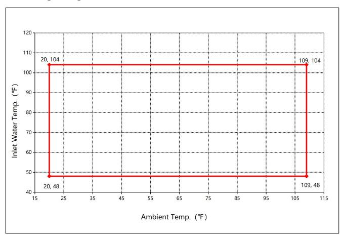
**Note:** Please make sure that the swimming pool heat pump operates within the ambient temperature and water inlet temperature range, as the figure shows. If the unit operates outside the temperature range, damage may occur.
