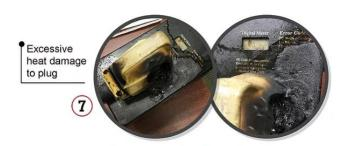
A poor connection forces the voltage to arc creating extreme heat which can result in extreme melting.
