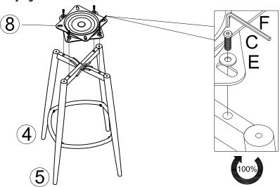
5 Turn assembled legs in step 3 upside down, and attach them to seat (1), using bolts (C), flat washers (E) and allen wrench (F). Note: Tighten all bolts.
