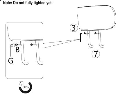
Attach the assembled backrest part in step 6 to seat part (1), using bolts (B), allen wrench (G). Fully tighten all the bolts.
