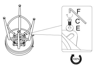
Attach the circle seat part (2) to seat part (1), using bolts (C), flat washers (E), allen wrench (F). 6 Attach parts (7) to backrest part (3), using bolts (B), allen wrench (G). Fully tighten all the bolts.
