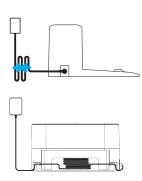
3. Connect the adapter to the charging base and arrange the power cable properly.
