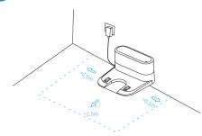
4. Place the charging base in proper position and power on for charging.
