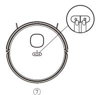
Press both "Power + Charge" buttons for 3 seconds and the light starts to flash, which means the robot starts network distribution.
