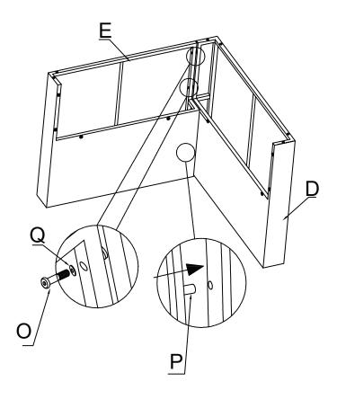
Do not fully tighten all bolts until assembly is complete.
