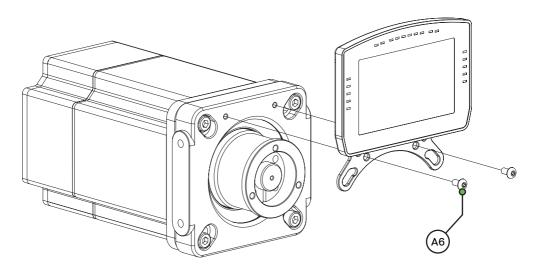
As for mounting directly onto your motor or older style front mount, this is very straightforward. Remove the existing upper bolts which hold the motor in place. Re-use these bolts and washers to fix the mounting bracket to the front mount.
