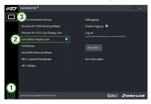
Tick the 'Activate' tickbox next to 'Grid DDU5 Display Unit' (2) and its icon (3) should appear on the left side of the screen. Selecting the icon (3) will take us to its device pages.
