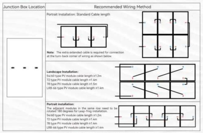
Figure 2 Junction Box Style and Wiring Method
