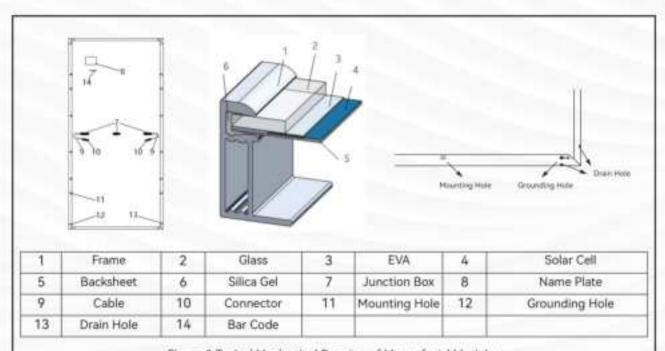
Figure 1 Typical Mechanical Drawing of Mono-facial Modules
