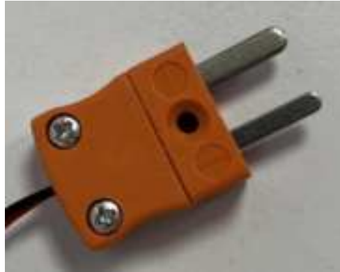
Figure 2 Thermocouple end of Element-B connection cable
